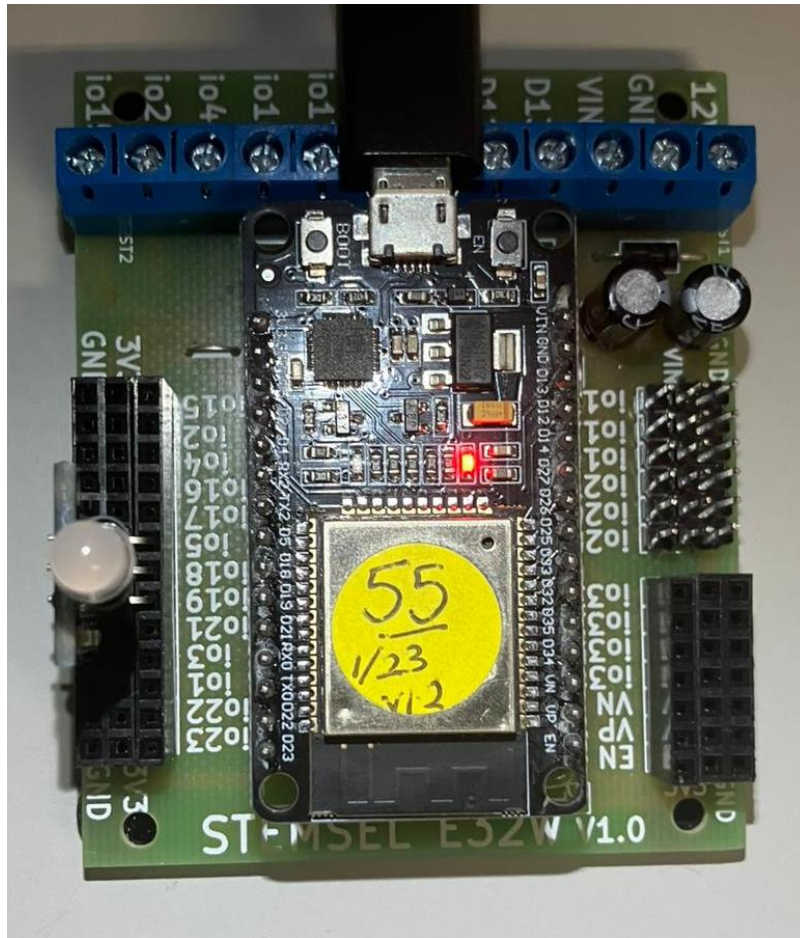
Figure 7: Circuit board connection with I/O parts (top view)
